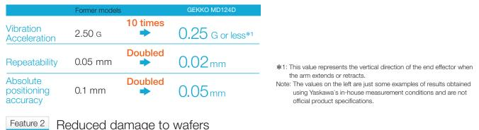
The SEMISTAR-GEKKO series has achieved low vibration, resulting in the adoption of a passive grip end effector. This minimizes stress on a wafer, enabling high-speed and high-accuracy wafer transfers with less damage to wafers.
